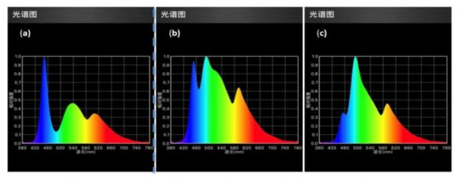
Remarks: (a) Ordinary diffuser plate + LED display spectrum chart; (b) Eye protection QD board (banburying) + LED display spectrum chart, Quantum dot concentration, QD Board thickness; (c) Eye protection QD board (banburying) + LED display spectrum chart, Quantum dot concentration, QD Board thickness.
