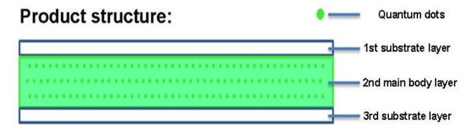
**Technological process :** quantum dots production  $\rightarrow$  formula debugging granulation  $\rightarrow$  extrusion molding  $\rightarrow$  Board processing and testing
